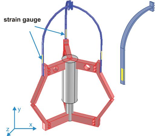
Fig. 5. RCC gripper with force sensing
