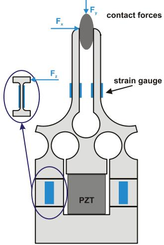
Fig. 3. Modified micro-gripper with force sensing
